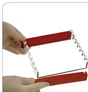
Casting dams allow gels to be rapidly cast externally while the unit is in use for gel running
